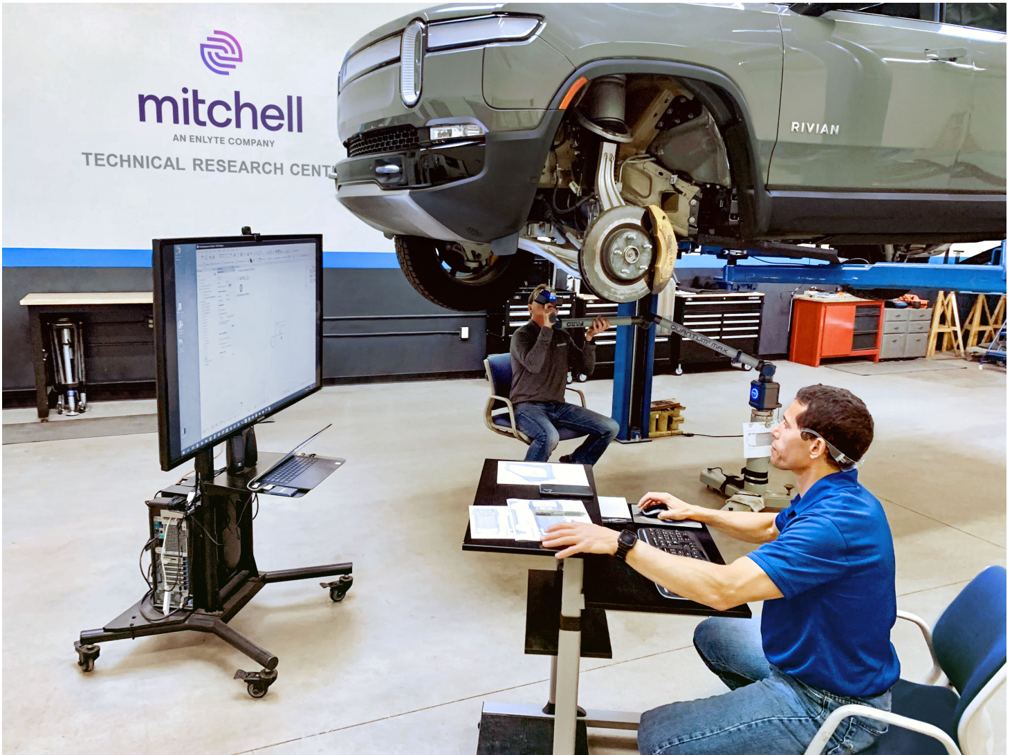
Mitchell employees collect 3D measurements and scans on the Rivian R1T at the company's Technical Research Center in San Diego.
